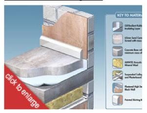
Before installing a floating screed, the G8 sound insulation must be laid with the BACKING FABRIC UPPERMOST with the joints overlapped by 50mm and lapped up the walls high enough to contain the screed. Usually about 20cm. Duct tape can be used to facilitate this.
