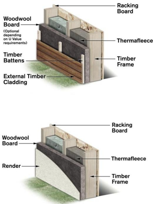
Unlike traditional timber frame systems, the racking board is positioned to the inside of the timber frame. The external insulation attached to the timber frame maintains the frame above the dewpoint temperature reducing the risk of condensation.
