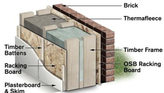
The twin frame system ensures that no thermal bridging occurs within the construction helping to maximise insulation performance. By using two 89mm structural timber frames, the width of the construction can be varied to achieve specific insulation performance.
