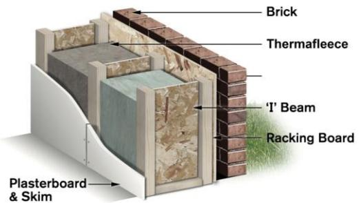
A service void can be created by counter battening along the timber frame internal face and fixing the internal finishing board. This ensures that the insulation remains undisturbed and airtightness remains intact when services are accessed for maintenance. The insulation performance of the void can be improved by installing an Eden Low Emissivity Membrane against the insulation.
