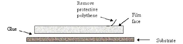
NOTE. Some of our film faced material has a polythene film protecting it. This film should be removed prior to installation otherwise the sound absorption of the product will be adversely affected.
