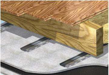
we supply, the bars will create an effective acoustic break between the bottom of the existing joists and the ceiling. If not fitted directly beneath the floor joists, Sound Reducing Resilient Bars can be supported by 50mm square battens screwed to the underside of any existing ceiling.
