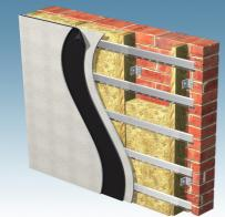
If you are experiencing loud noise such as music from the other side of a wall, we recommend using the soundproofing mats with our resilient bars and Acoustic Plasterboard. The soundproofing mat is sandwiched between two layers of the plasterboard which in turn are screwed into the bars which are supported by insulated timber stud. See our Resilient Bar information for more details.
