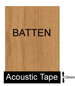
The Acoustic Tape does not replace the need for decoupling the wall with the Resilient Bar but does help greatly increase the walls performance against low frequency bass vibration.
