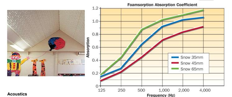
The special open face profiled foam pattern is the main reason why Foamsorption tiles outperform other acoustic tiles. This leads to higher sound absorption in buildings resulting in greater reduction of reverberant noise.
