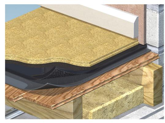
QuietBoard installed on top of our Acousticel R10 resilient insulation (As shown left) provides a very efficient and stable floating floor.
