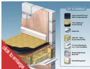
R10 is supplied in rolls which are unrolled and laid on the floor wall to wall with the edges butt jointed.
