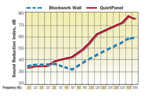
Composition 15mm noise blocking layer laminated to 12.5mm non-flammable, high density sound blocking acoustic panel.
